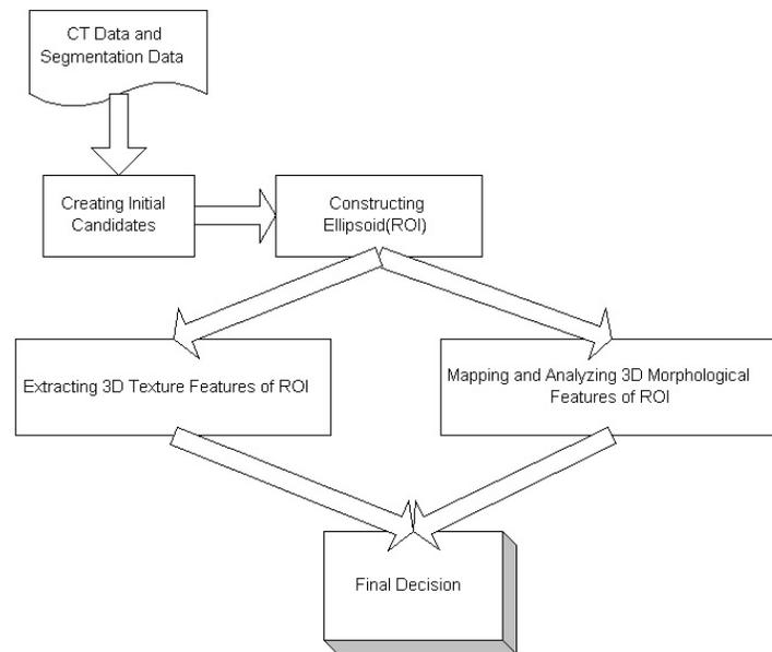
Figure 1: Flowchart of the presented CAD Method.
