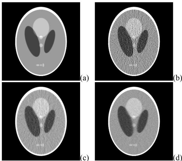
Figure 1: Transversal slice of the modified 3D Shepp-Logan phantom: (a) noise free image, (b) noisy image by FBP with the Ramp filter, (c) FBP image with the Hanning filter, and (d) FBP image from the KL-PWLS smoothed sinogram.
