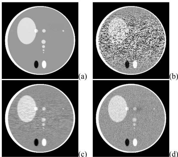
Figure 2: Sagittal slice of the modified 3D Shepp-Logan phantom: (a) noise free image, (b) noisy image by FBP with the Ramp filter, (c) FBP image with the Hanning filter, and (d) FBP image from the KL-PWLS smoothed sinogram.
