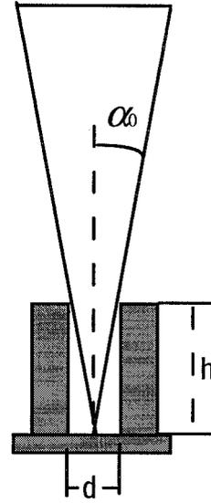
Fig. 2. For a specific collimator, the arriving photons on the crystal can be represented as all the emissions from the fan region.
