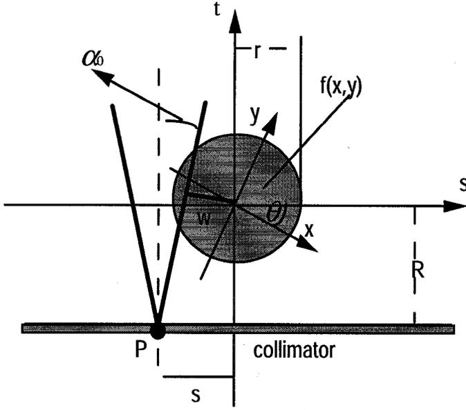
Fig. 1. The radionuclide distribution  $f(x,y)$  is located in the disc  $B(r)$ , the collimator is away from the origin at a distance  $R$ . The total photons through the collimator hole  $P$  is an integral inside the fan-like region.
