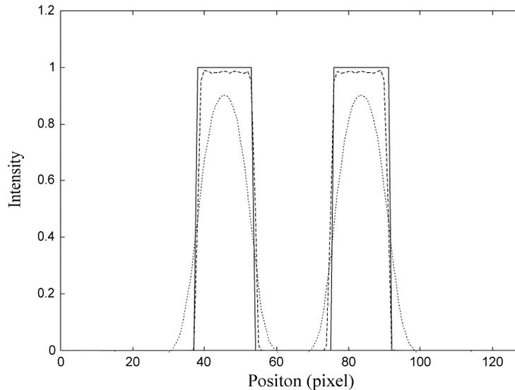
Fig. 6. Profiles of the images presented in Fig. 5 along the central horizontal line. The solid, dotted, and dashed lines represent profiles for the phantom, the reconstructed image without compensation, and the reconstructed image with compensation using kernel matrix method, respectively.
