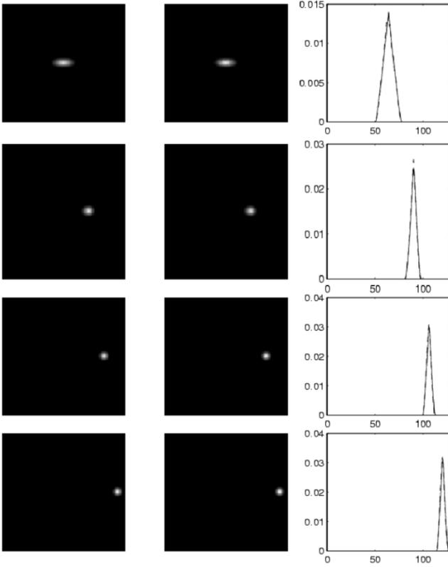
Fig. 3. Comparison of calculated geometrical PSF (left column) with Monte Carlo simulation (middle column) at depth 35 cm and offset of 0, 5, 10, and 15 cm, respectively (from top to bottom). The right column shows the profiles through the center of the geometric PSF, with the theoretical calculation in the solid line and the Monte Carlo simulation in the dashed line (1 pixel = 0.3438 cm).
