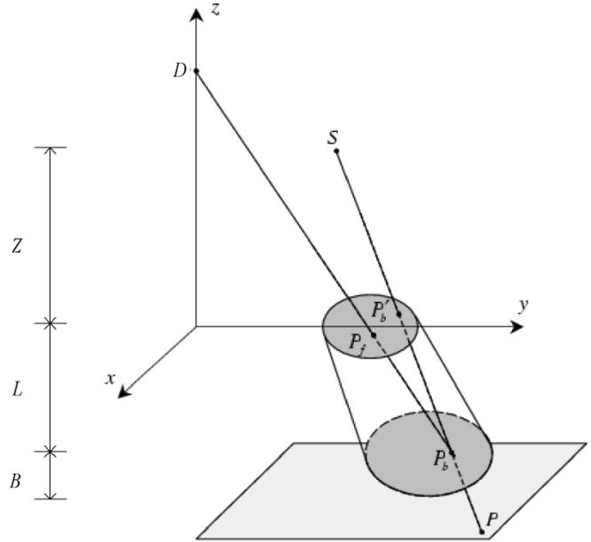
Fig. 2. Geometrical model for the point-spread function of VFF collimators. Point source is located at a distance  $Z$  from the collimator face.  $L$  is the collimator thickness, and  $B$  is the distance between the collimator backplane and the image plane inside the scintillation crystal.
