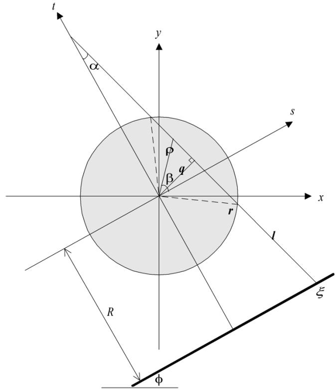
Fig. 4. Projection ray  $l$  in polar coordinate system:  $\rho \cos(\beta - \alpha) = q(\xi)$ ,  $\beta \in (\alpha - \gamma, \alpha + \gamma)$ , where  $\gamma = \cos^{-1}(q(\xi)/r)$  and  $r$  is the radius of the object support.
