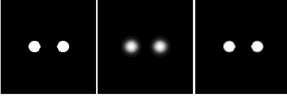
Fig. 5. Fan-beam collimated SPECT studies on reconstructed images, where the focal length  $D = 200$  pixel units. From left to right are the original phantom, the reconstruction image without detector response compensation, and the reconstructed image with compensation using kernel matrix method, respectively.
