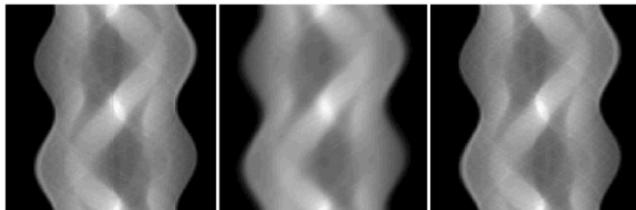
Fig. 8. VFF collimated SPECT studies on sinograms, where  $D(\xi) = a + b|\xi|$ ,  $a = 150$  pixel units, and  $b = 2.5$ . From left to right are the ideal sinogram from the Shepp-Logan phantom, the simulated collimator blurred sinogram, and the corrected sinogram using our kernel matrix method.
