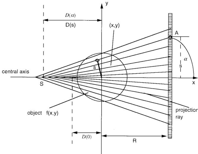
Fig. 1. Spatially varying focal length fan-beam geometry.
